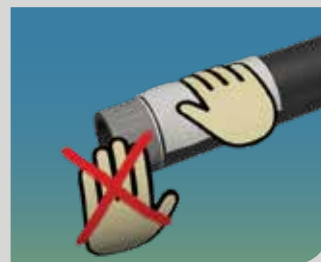
3. Do not touch the scraped area with bare hands after scraping and cleaning
